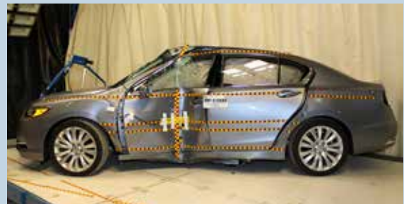
The left side of a vehicle after crash testing. Simulation can be used to minimize the number of physical tests needed. Image courtesy of National Highway Traffic Safety Administration.
